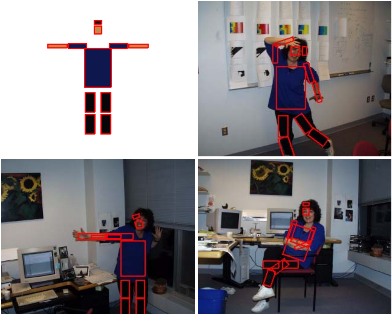
Figure 4: Recognition results using the person model. The top left image shows the model, which has revolute joints, in its default configuration. The remaining three images show examples of the globally best matching configuration.
