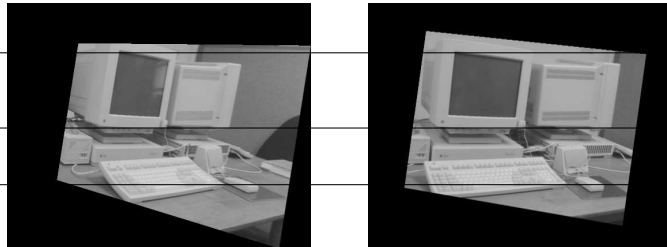
Rectified images - epipolar lines horizontal. Can be fused if superimposed in red and green and viewed through filtered glasses.
