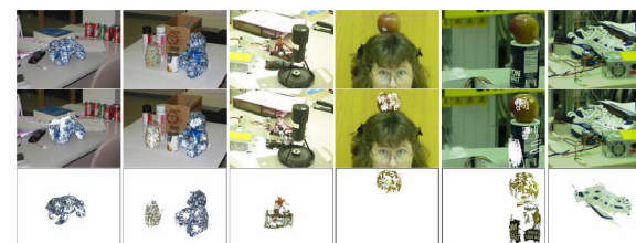
Figure 3: Object recognition experiments. The three rows of this figure show (respectively) input images, model patches matched to these images, and recognized models rendered in their estimated pose. Note that the teddy bear in the leftmost column is in a pose quite different from those used to acquire its model. Also note the significant amount of clutter and occlusion in each image.
