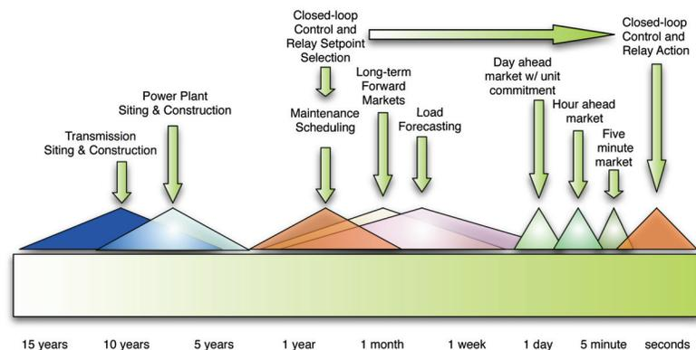
Figure 1. Representative decision-making time scales for electric power systems.
