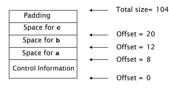
Within **p**, each local data object is addressed by its offset relative to the start of the frame.
