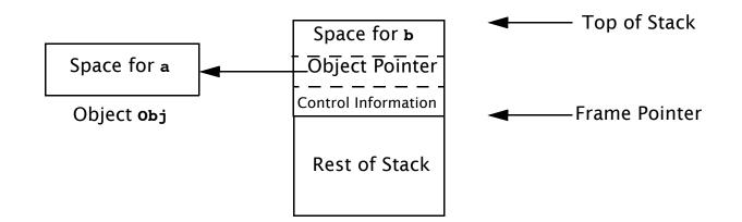
When **a+b** is computed, **b**, a local variable, is accessed directly through the frame pointer. **a**, a member of object **obj**, is accessed indirectly through the object pointer that is stored in the frame (as all parameters to a method are).
