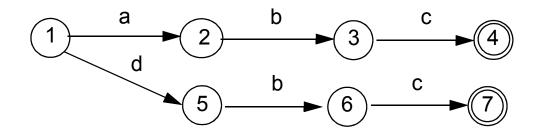
Initially we have a merged nonaccepting state {1,2,3,5,6} and a merged accepting state {4,7}.
