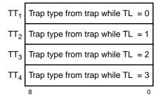
Figure 23—Trap Type Register
