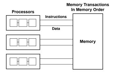
Figure 43—Data Memory Paths: Multiprocessor System
