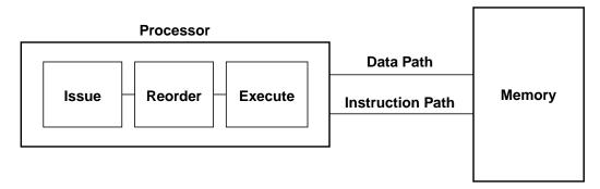
Figure 42—Processor Model: Uniprocessor System
