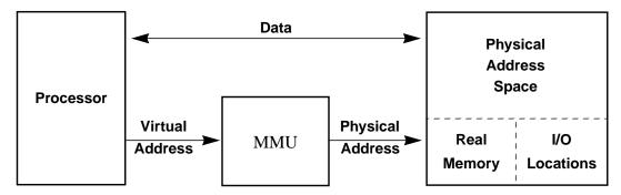
Figure 48—Logical Diagram of a SPARC-V9 System with an MMU
