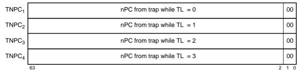
Figure 21—Trap Next Program Counter Register
