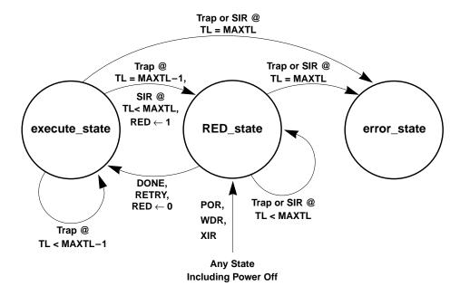
Figure 37—Processor State Diagram
