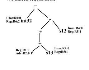
We now work *upward*, considering operators whose children have been labeled. Again, if an operator can be generated by a nonterminal, we mark the operator with the nonterminal, the production used to generate the operator, and the total cost (including the cost to generate all children).
