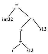
We match tree nodes bottom-up. Each node is labeled with the nonterminals it can be reduced to, the production used to produce the nonterminal, and the cost to generate the node (and its children) from the nonterminal.
