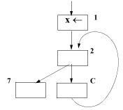
We isolate and reduce the while loop formed by  $b_2$  and  $b_C$ , creating  $b_{W^*}$ . The transfer function is
