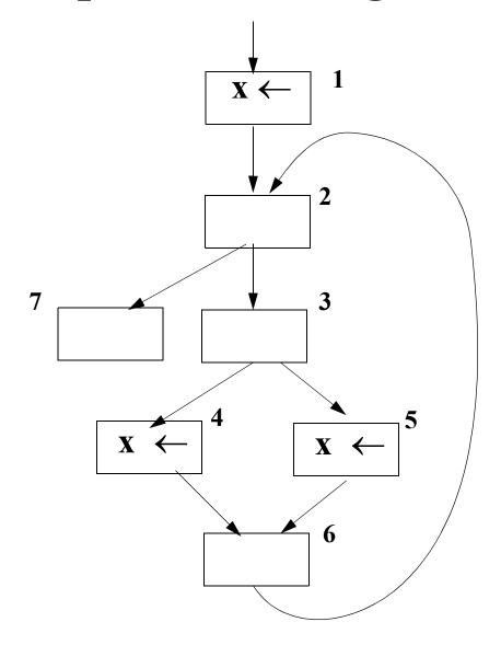
The transfer functions are either constant-valued  $(f_1=\{b1\}, f_4=\{b4\}, f_5=\{b5\})$  or identity functions  $(f_2=f_3=f_6=f_7=Id)$ .
