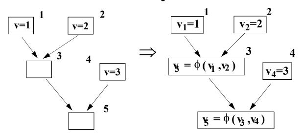
Now, DF(b1) = {b3}, so we add a phi function in b3. This adds an assignment into b3. We then look at DF(b3) = {b5}, so another phi function must be added to b5.
