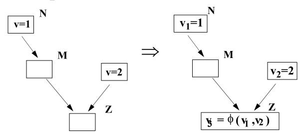
Here, (N dom M) but  $\neg$ (N sdom Z), so a phi function is needed in Z.
