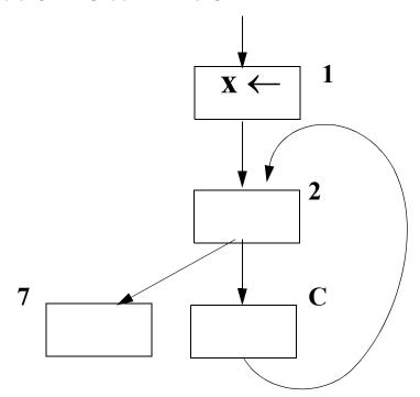
We isolate and reduce the while loop formed by  $b_2$  and  $b_C$ , creating  $b_W$ . The transfer function is
