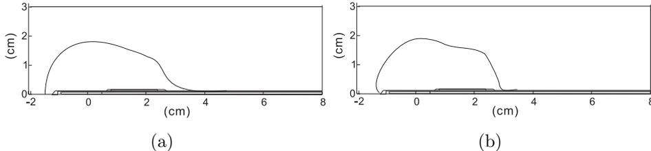
**Figure 5.** Comparing simulated  $Q(\mathbf{r})$  profiles using the average dielectric properties (43.03,1.69). (a) antenna design presented by Yang et al. (b) optimal design derived by our algorithm
