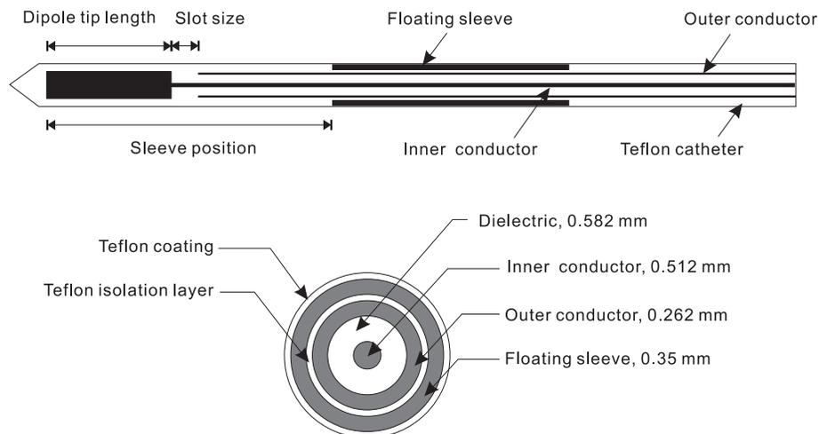
**Figure 1.** Structure of the floating sleeve antenna. Wall thicknesses of fixed dimensions are labelled in the figure.
