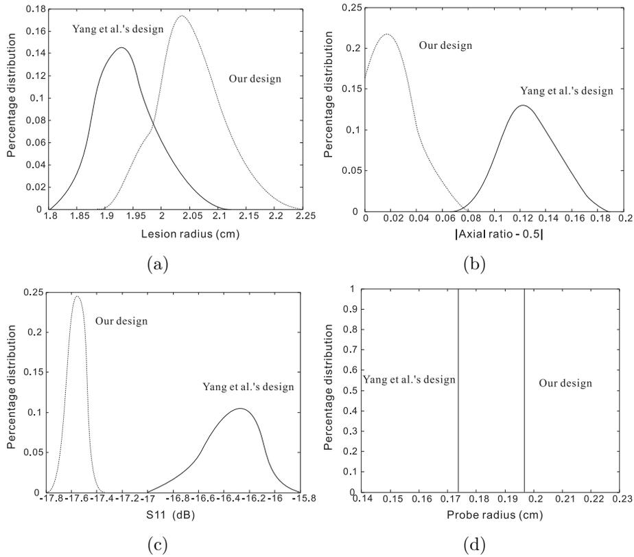
**Figure 4.** Variations of individual objective metrics (frequency plot). (a) Lesion radius, (b)  $|\text{Axial ratio} - 0.5|$ , (c)  $S_{11}$ , (d) Probe radius
