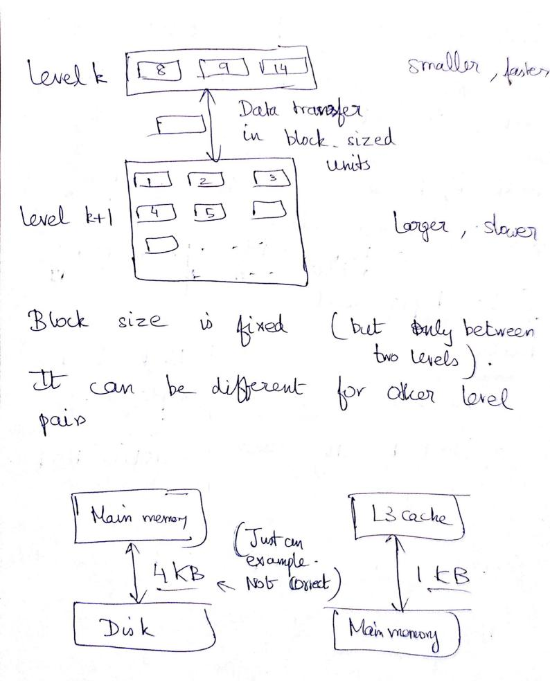
Then -> level k fetches d from level k+1, and it will store it. K DODD What if k is full? Remove some old block and put DDDD d there Cache Replacement Policy Block to be o Random replaced victim block. · Least Recently Used Blig. Arrays Vs Linked Lists. suppose -> linear search. Good spatial locality?
