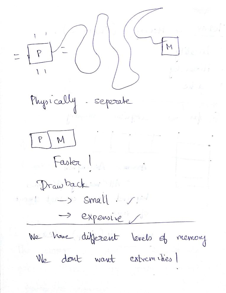
Processor LO Registers LI /LI Cache L2/L2 (ache) laster expensive L3/L3 cache L4 / Main Memory larger 15/ Disks (Local 1 slower Web (Cloud) ... cheaper. Access times O cycles Register no 1 to 30 cycles. Cache ~ Main Memory ~ 20 ~ 200 cycles. 10's of millions of Disk cy cles The closer your douba gets to the processor, the faster your program is going bo execute.
