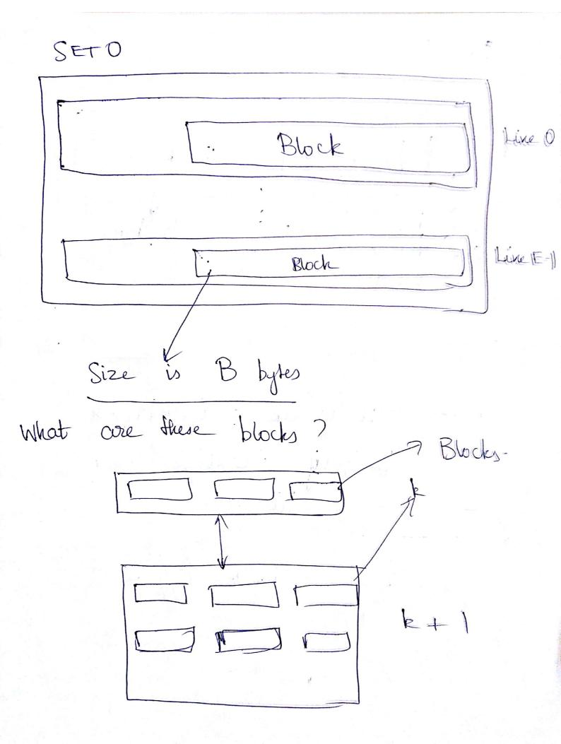
Set 0 Tag bits Block Valid bit B bytes 0 -> Not Valid 1 -> Valid It is like a identifier Uniquely identifies each line. Structure //. Basic
