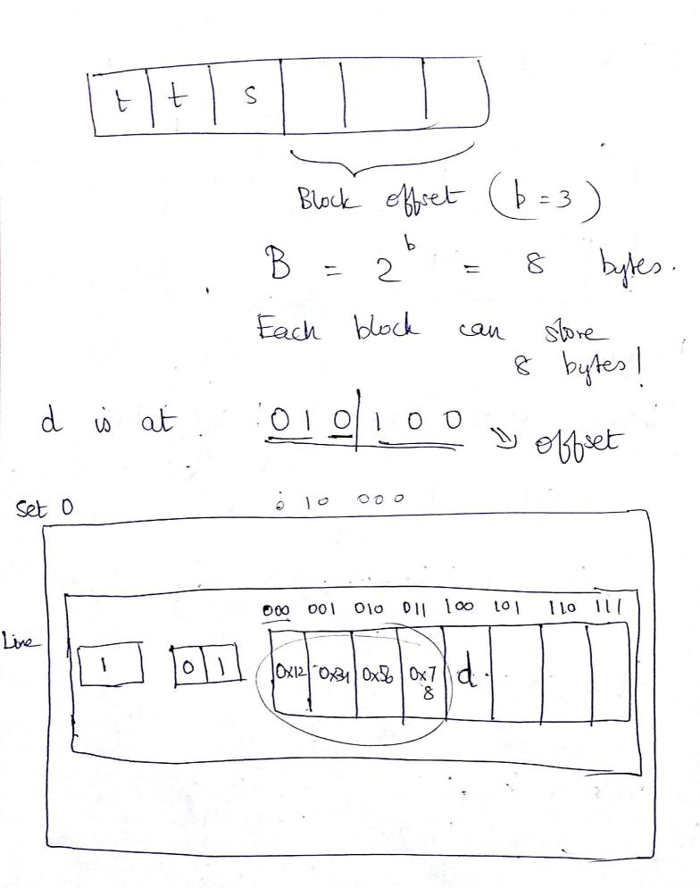
Suppose we want to access an at 01000 integer X Read 4 types starting at offset Suppose there is no line with the tag bit we were booking for ! Cache miss. Read the relevant data block from (k+1) and we evict / replace an existing line. The valid bit is not set (=0) then exict that line. (Simple) -> It all lines have valid bit set (=1), use a replacement policy.
