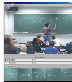
Figure 7: Screen shot from a region-based playback program. The top image shows the video being played, and the bottom part shows all the regions in the video.
