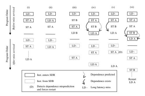
Figure 4 Examples showing various hazard conditions handling in SRL.
