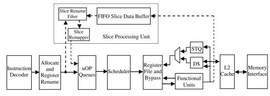
Figure 1 Block diagram of a CFP processor
