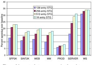
Figure 2 Impact of store queue size for a latency tolerant processor.
