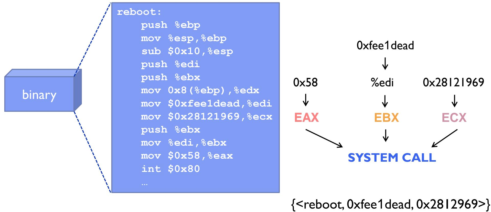
We parse an input binary, locate system calls and wrapper function calls, and employ dataflow analysis.
