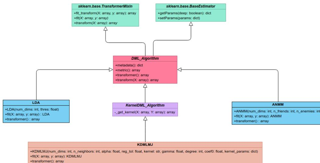
Figure 13: Class diagram of the algorithms developed in `pyDML` (only `LDA`, `ANMM` and `KANMM` are shown, but the rest of the algorithms follow a similar structure, overriding the `metric()` or `transformer()` method, depending on how the algorithm has learned).
