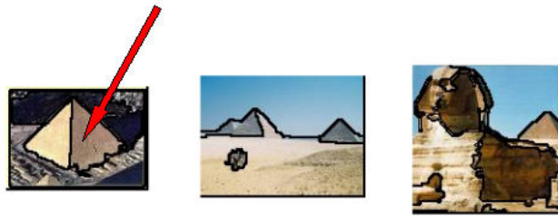
Figure 2: The image selection process on three retrieved images for the word “pyramids.” Segmentation boundaries are overlaid on the images. The region closest to the centroid of the largest cluster is indicated by the arrow, and that image is selected as the best for the word.
