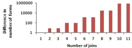
Figure 5: Comparing FormGen and the modified FormGen algorithm that eliminates duplicates, for the DBLife schema. The number of maximum joins is shown on the X-axis. The Y-axis shows the difference in the number of forms on the \log scale. The new approach generates 30-40% fewer forms.
