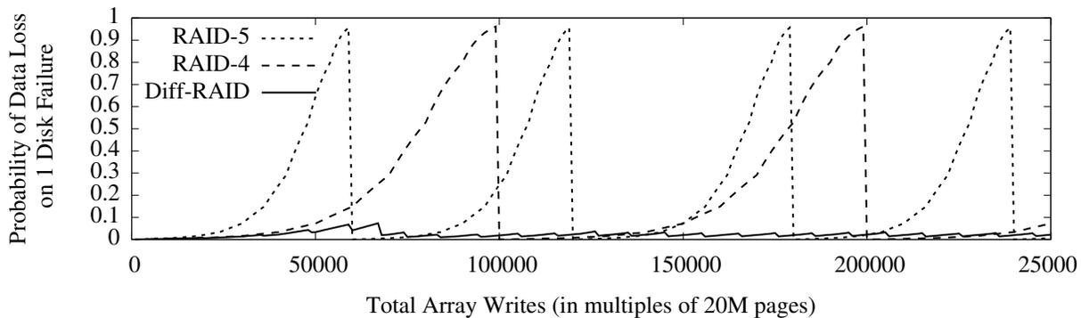
**Figure 3: RAID-5 and RAID-4 versus Diff-RAID for a 6-device array. Diff-RAID is configured to use a RAID-4 parity assignment – (100, 0, 0, 0, 0, 0) – but differs by performing age-driven shuffling on device replacements.**
