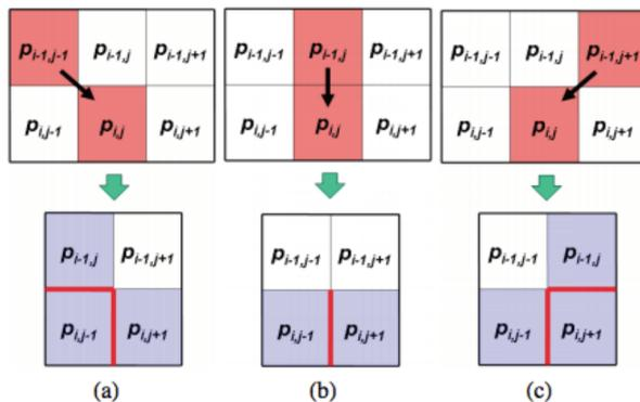
Figure 1: Illustration on neighborhood changes after seam removal
