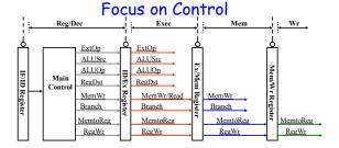
The Main Control generates the control signals during Reg/Dec
