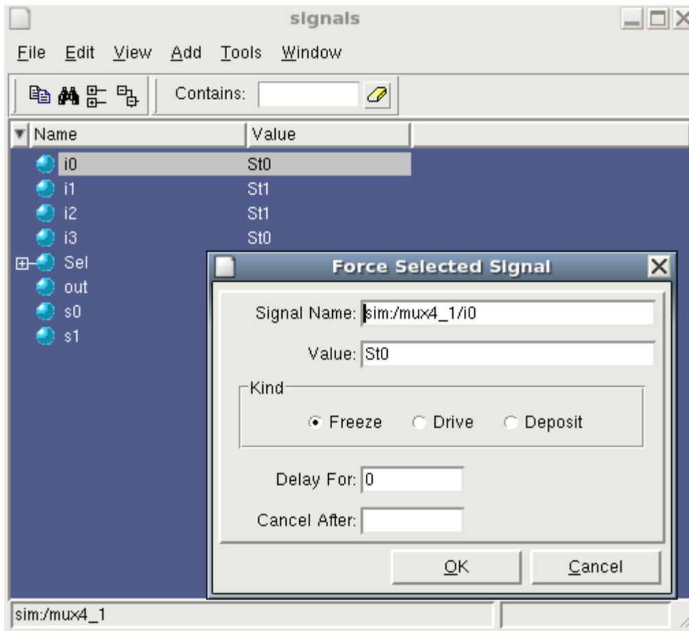
**Figure 3 - Forcing signals in ModelSim**
