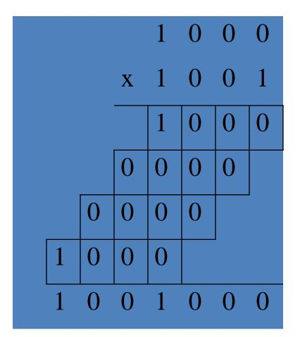
Adding all partial products simultaneously using an array of basic cells
