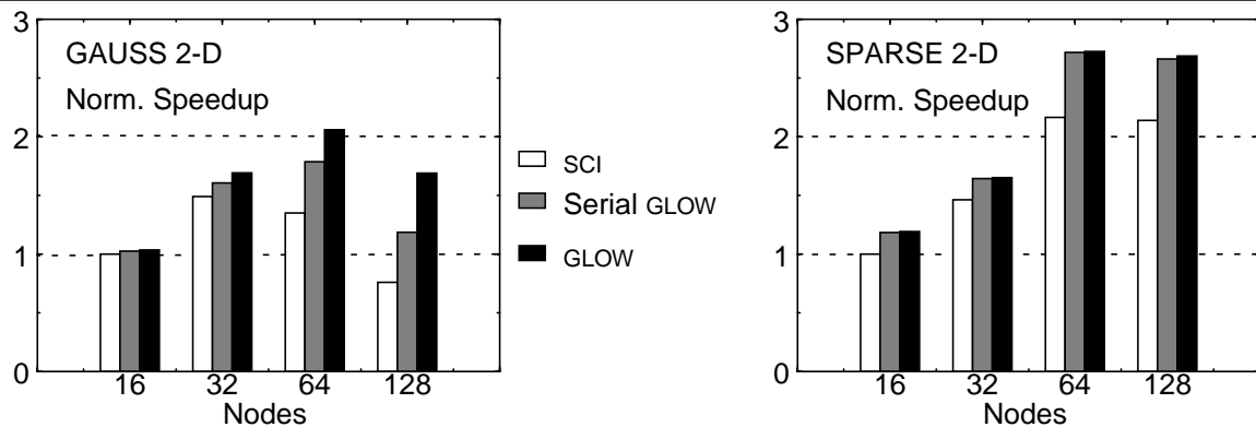
Figure 4.11. Normalized speedup for GAUSS and SPARSE with serial GLOW. Base system is SCI on 16 nodes.
