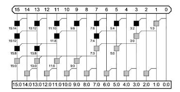
The configuration of a 16-bit Ladner-Fischer adder is shown in the above diagram. The P/G signals from Bit 0 to the odd bits are generated by a tree. This tree is not exactly a binary tree, because it adds some nodes to generate the P/G signals of the intermediate bits. Then the P/G signals from Bit 0 to the even bits are generated by the final stage according to the P/G signals of the odd bits.
