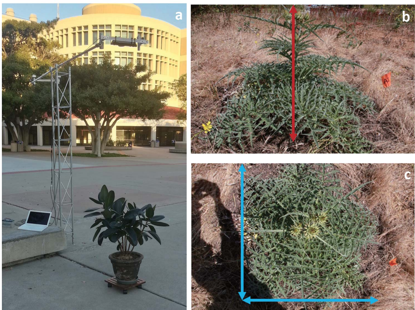
Figure 1. (a) The “tower mode” experimental setup used for nadir measurements with Kinect (see Sections 2.3 and 2.4). (b) Side view and (c) nadir view of a wild artichoke plant recorded during the field test (see Section 2.4). Blue and red lines represent plant’s basal diameter and height as measured manually with a ruler.
