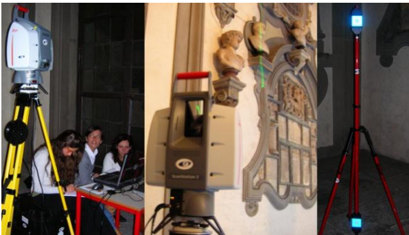
Figure 2: Leica ScanStation2 setup and Reflective targets used to align multiple scans.
