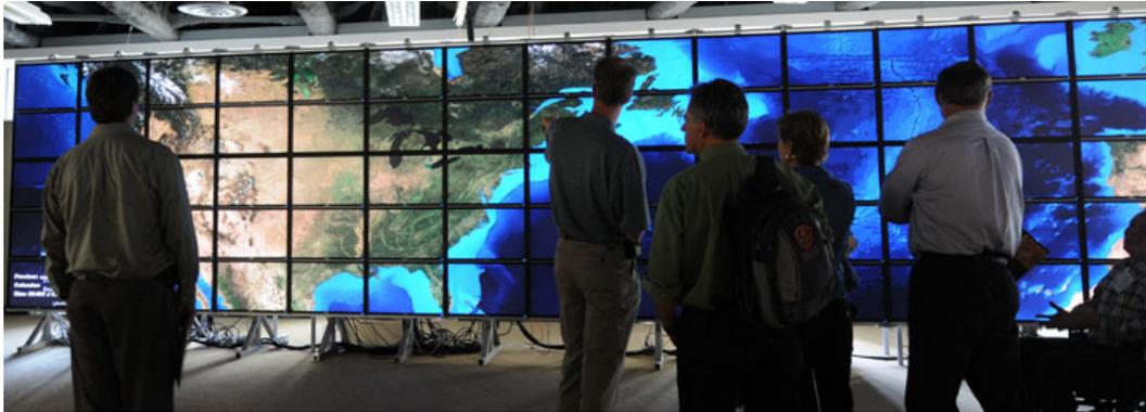
**Figure 2.1:** Users viewing a time varying version of NASA's 44 giga pixel Blue Marble Next Generation data set [SVS<sup>+</sup>05] on a 286 million pixel resolution display
