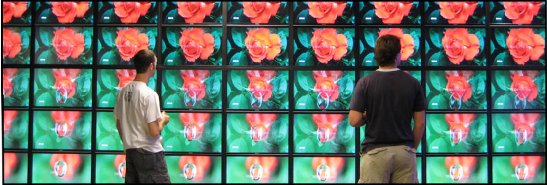
Figure 4.1: The system displaying BBC’s HD In Full Bloom video of time lapse photography [bbc]. Each of the 70 monitors shows a temporal offset of a single video frame.
