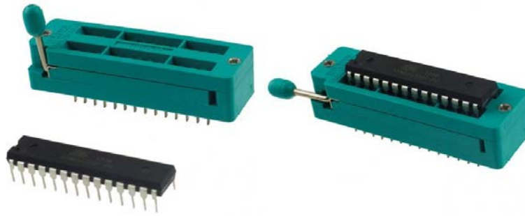
Figure 7: Left shows ZIF socket before IC insertion. Right shows ZIF socket after IC insertion
