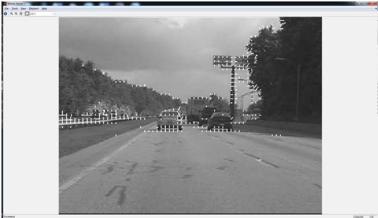
The frame from doing OF on global motion analysis shows where each object is moving. OF shows that the movement vector of each object in the frame is pointing upward means that the camera is moving to face downward.
