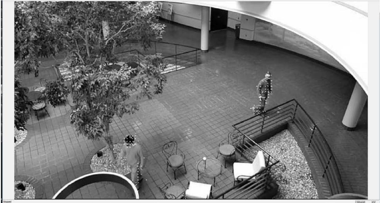
The frame from doing OF on block-based motion analysis shows the direction of where each block is moving. Knowing where each block moves will help approximate its location in the new frame. The video can be encoded by keeping track of the blocks and its motion vector, then moving the block along its motion vector to generate the next frame.
