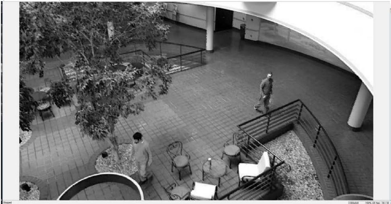
The frame from doing DFD on pixel-based motion analysis appears to be blurrier because it only uses pixels from the previous frame to approximate each pixel among their neighboring pixels. Looking closely at the man on the right or the pillars will reveal that some pixels are a little out of place, which makes the man look blurry.
