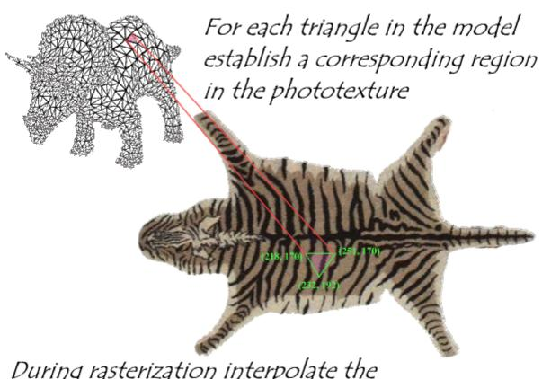
During rasterization interpolate the coordinate indices into the texture map
