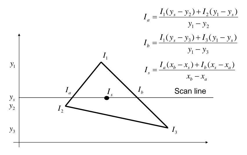
Replace I to uw, vw, and w, then compute (uw/w, and vw/w)
