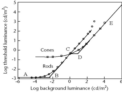
**Figure 1:** The TVI function (adapted from <sup>6</sup>). To integrate equation 5 analytically, we use approximation by linear segments AB, BC, CD, and DE.
