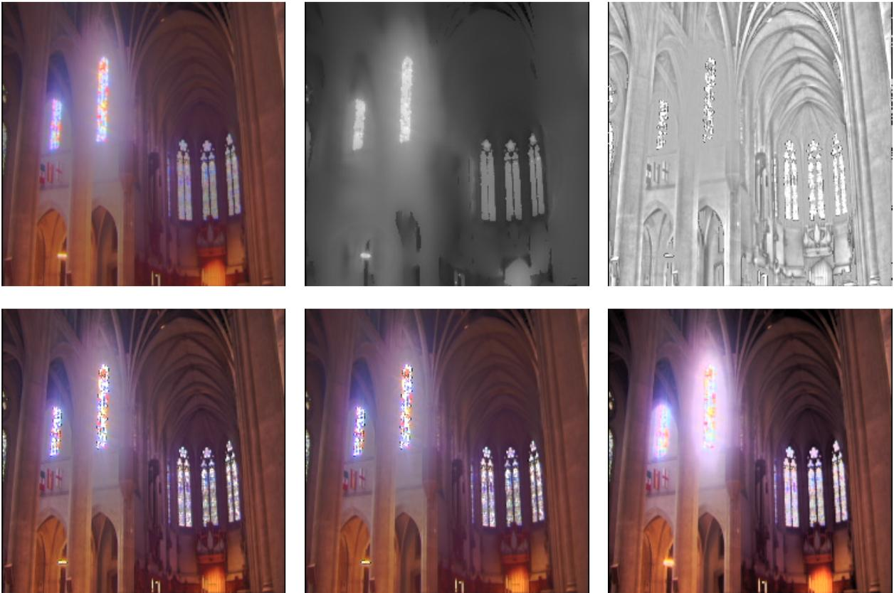
**Figure 3:** Operation of our algorithm. In reading order: a. application of  $TM(L)$  to pixel luminances, b. computed adaptation image after tone mapping by  $TM$ , c. details image (midlevel grey corresponds to value one), d. final result using equation 2, e. same using visible contrast definition (equations 3 and 4), f. histogram-based tone mapping<sup>11</sup> result.
