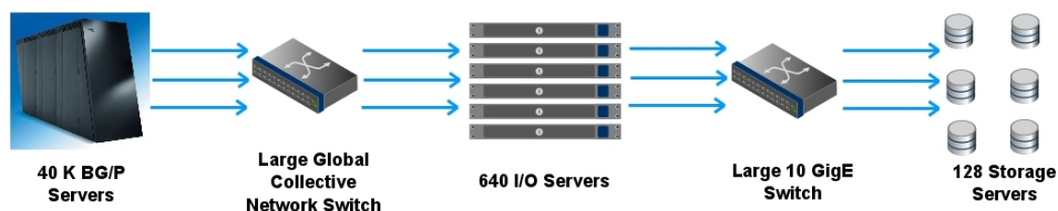
Fig. 2. Intrepid Supercomputer and GPFS. 40 BG/P racks redirect I/O requests over a specialized network to 640 I/O servers, which in turn use a large 10 GigE switch to access 128 storage servers.
