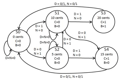
b. How many **flip-flops** (storage elements) will be needed to implement the finite state machine designed in (a)? (1 Point)
