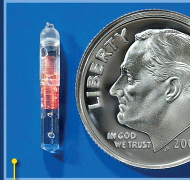
**SIZE** The device is 11 millimeters long and about 1 mm in diameter, comparable to a grain of rice.
