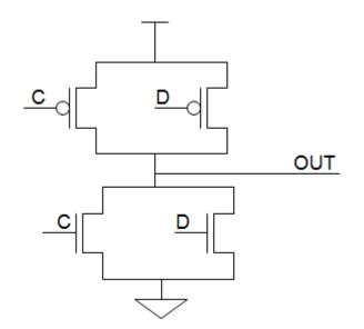
The circuit shown above (C and D are the inputs and OUT is the output) has a major flaw. What is it? *Hint*: Evaluate the circuit for all sets of inputs.
