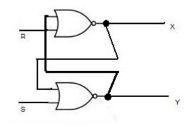
a. (2 points) For this RS latch, what are the values of X and Y, if S = 1 and R = 0? X = 1 Y = 0
