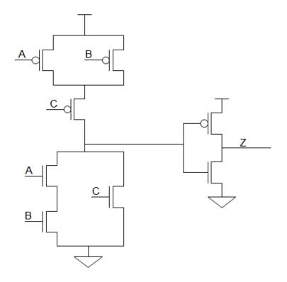
In the above circuit, A, B, and C are the inputs, and Z is the output.
