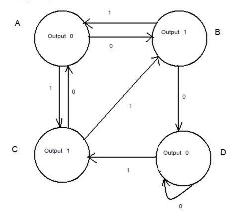
Assume that A is the start state in the FSM shown above. Determine the output sequence and the final state when the FSM acts on the input stream 111101.
