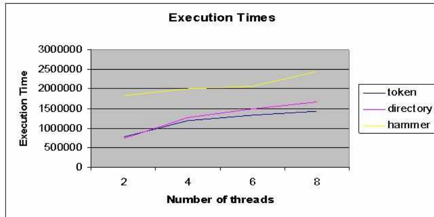
Figure 5: Execution times for bounded buffer with varying threads
