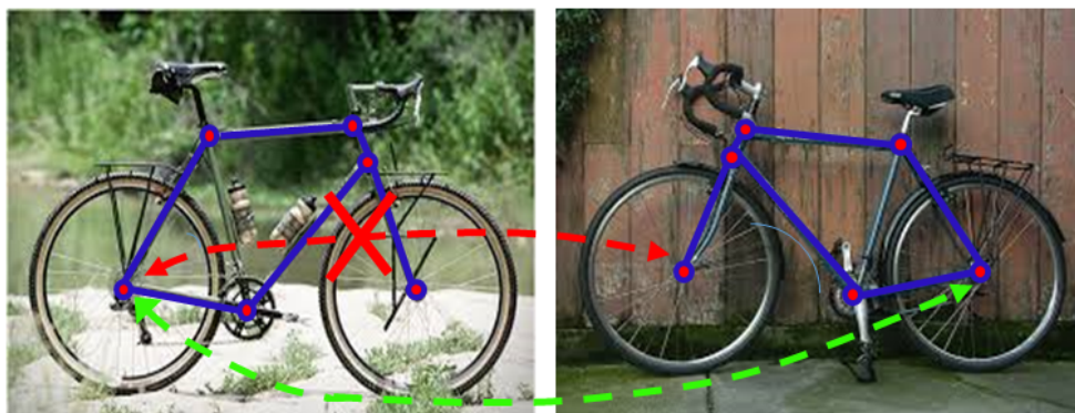
Figure 1.3: Pairwise assignment of interest points using second order geometric relationship.
