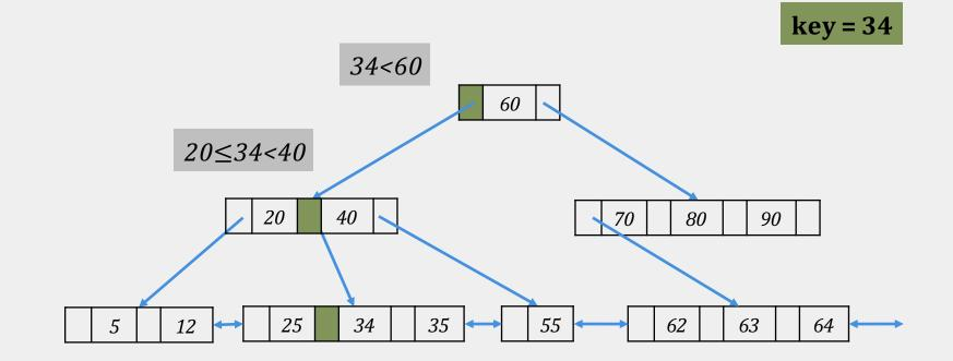
To locate the correct data entry in the leaf node, we can do either linear or binary search
