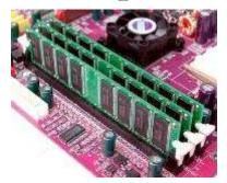
2. Multiple memory modules can themselves be aggregated by connecting to memory controller. (Data at Address A is in a specific memory module *k*)
