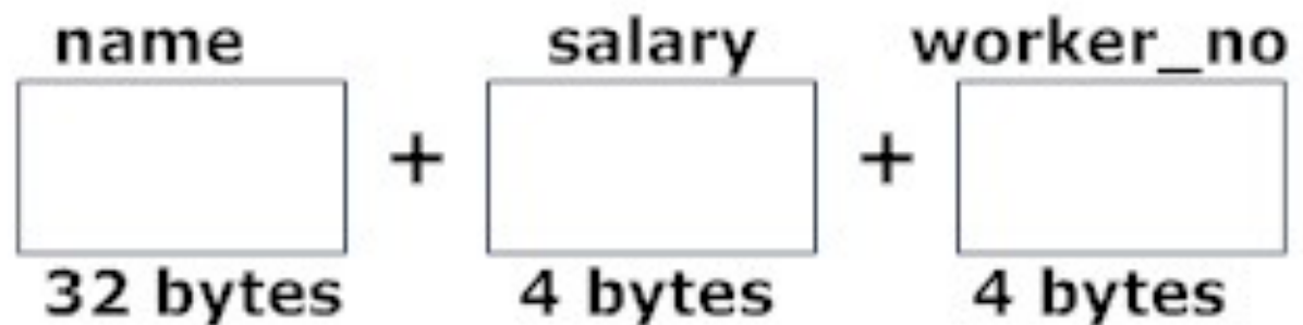
Fig: Memory allocation in case of structure
