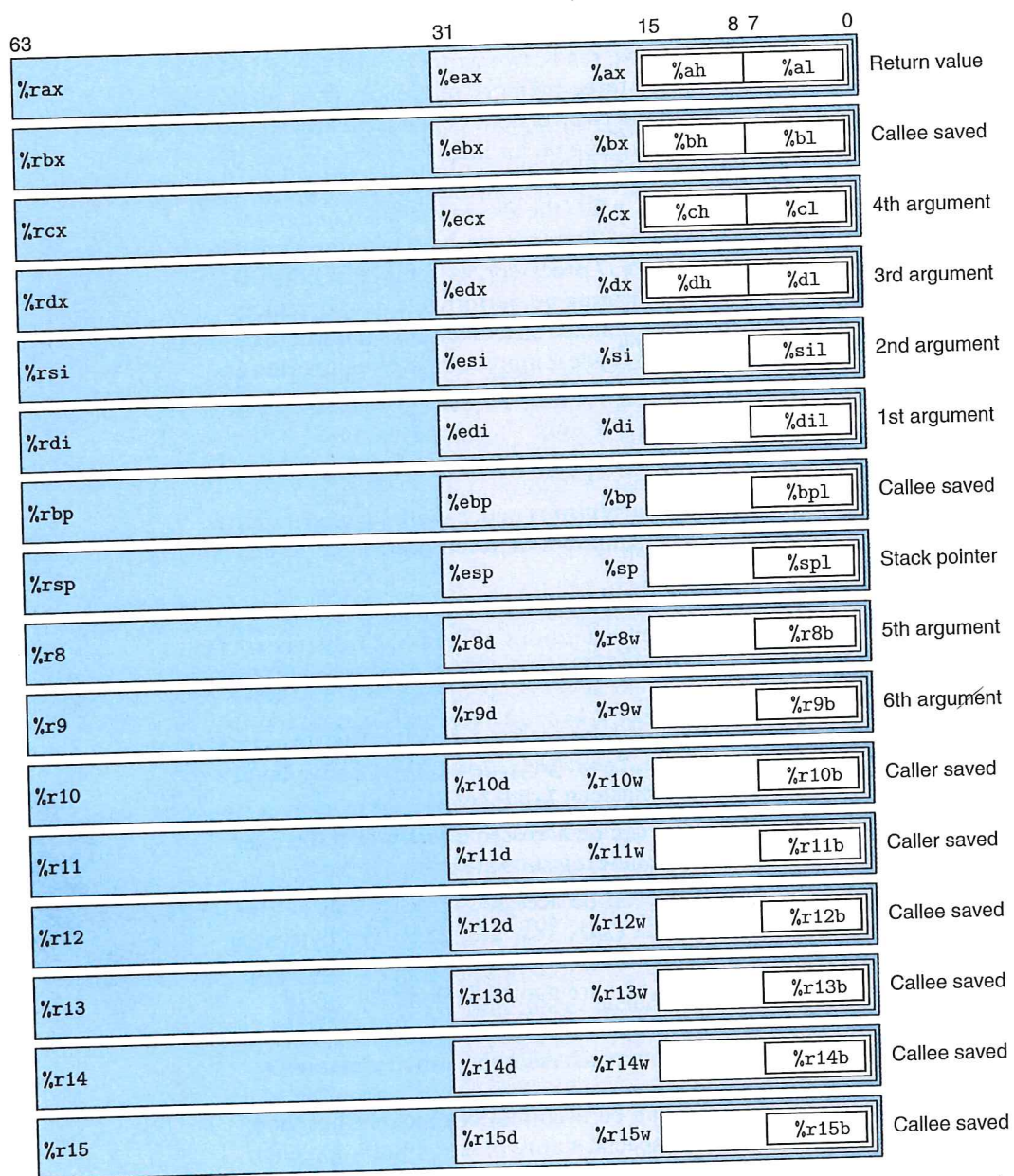
Figure 3.35 Integer registers. The existing eight registers are extended to 64-bit versions, and eight new registers are added. Each register can be accessed as either 8 bits (byte), 16 bits (word), 32 bits (double word), or 64 bits (quad word).
