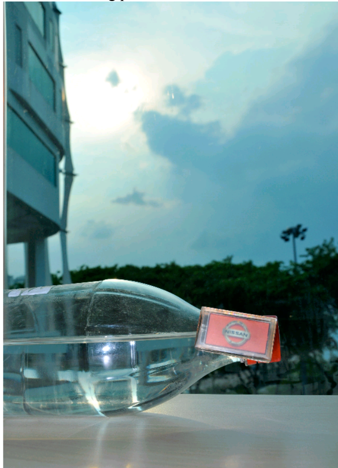
Fig 8: Device in Default state (when the device is not active) The NISSAN logo is replaced with full red to indicate “water not safe”.
