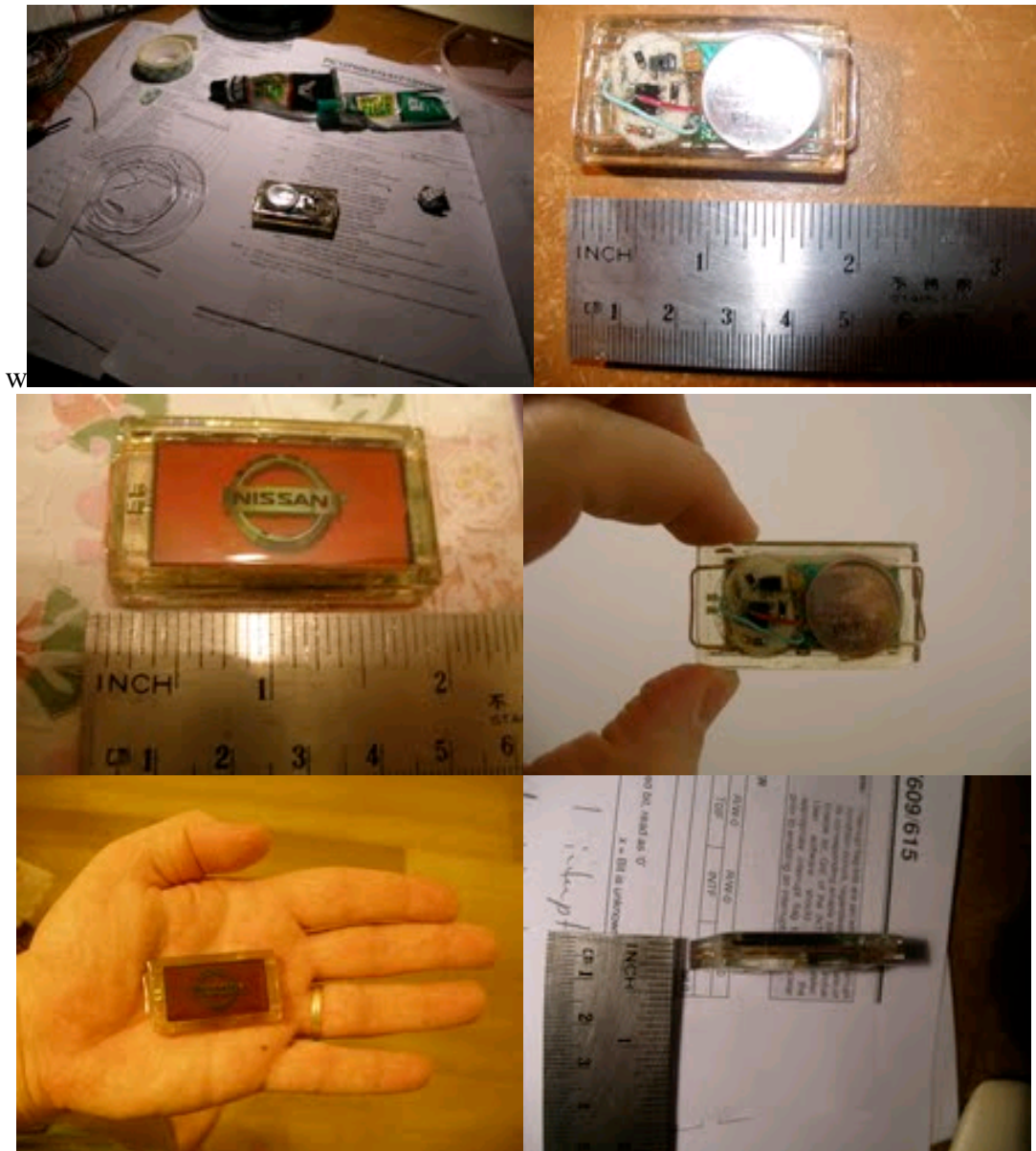
Fig 10 Assembly using SMD components embedded in epoxy. Notice the touch leads protruding outside.
