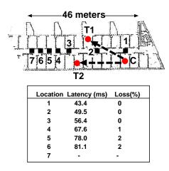
Figure 5: Floor-plan of building for MoB experiment scenarios. C is customer,  $T_1, T_2$  are traders (positions changed in different experiments as described in this section). The table indicates the latency and loss characteristics obtained in this environment using a source at C and destinations varying from 1-7 using Bluetooth.
