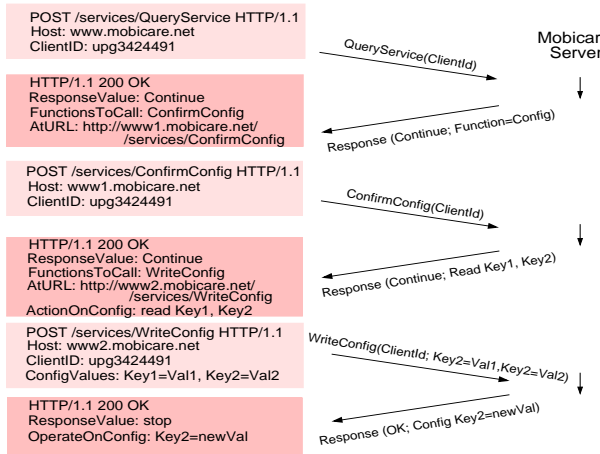
Figure 6: Configuration Service Protocol Exchange.
