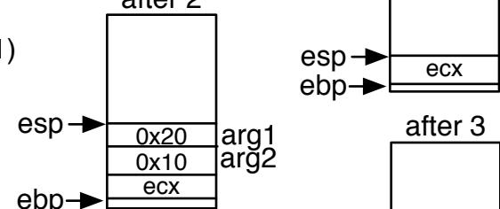
3. Call function (which pushes return address onto stack)
