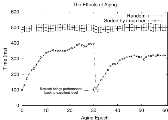
Figure 6: Undoing The Effects of Aging. The figure plots the total time to access 100 8-KB files within the same directory on the Linux platform. The upper line plots the time to access the files in random order, whereas the lower line sorts the files by i-number first. Along the x-axis, the age of the directory is increased; at every epoch, 5 random files are deleted, and then five new files are created. After 30 epochs, the directory is refreshed by copying its contents to a temporary directory, deleting the old directory, and then renaming the temporary directory.
