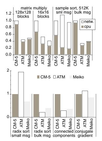
Figure 5: Comparison of seven Split-C benchmarks on the CM-5, the U-Net ATM cluster, and the Meiko CS-2. The execution times are normalized to the CM-5 and the computation/communication breakdown is shown for three applications.
