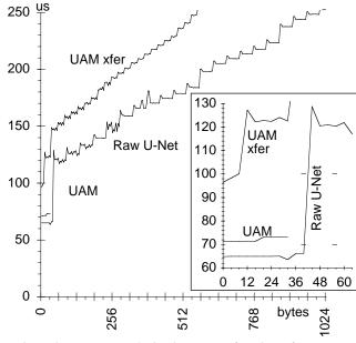
Figure 3: U-Net round-trip times as a function of message size. The *Raw U-Net* graph shows the round-trip times for a simple ping-pong benchmark using the U-Net interface directly. The inset graph highlights the performance on small messages. The *UAM* line measures the performance of U-Net Active Messages using reliable single-cell requests and replies whereas *UAM xfer* uses reliable block transfers of arbitrary size.
