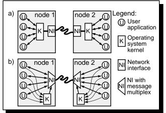
Figure 1: The traditional networking architecture (a) places the kernel in the path of all communication. The U-Net architecture (b) only uses a simple multiplexing/demultiplexing agent—that can be implemented in hardware—in the data communication path and uses the kernel only for set-up.
